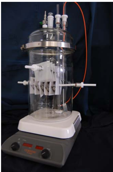
Figure 17: The simulated radiation environment vessel equipped with two Teflon hanging rods, ports for gas inlet and outlet, a safety pressure relief plug, and optional solution bubbler.
