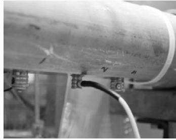
Figure 6. PulseEcho Transducer Mounted on the Instrument Spool Piece
