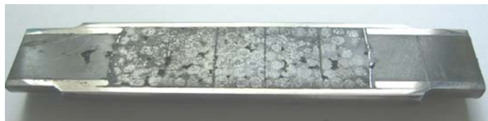
Bench scale mock-up of MAVR filled with lead
