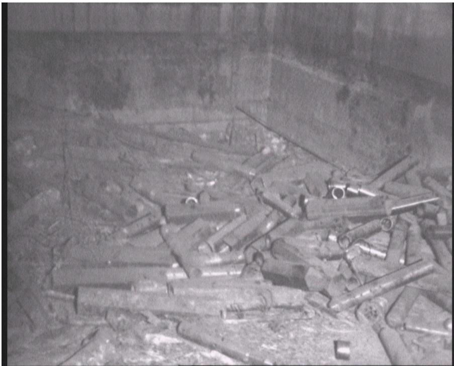
Fig. 2. Photograph from video survey showing the debris field – sub-assembly duct sections and lower ends
