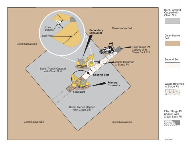
Figure 3. Test Pit Excavation Process
