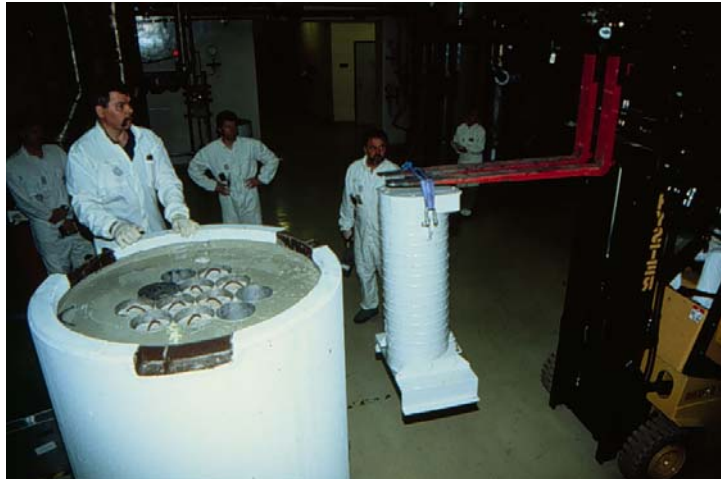
Fig. 4. Ion exchange column loaded into a concrete container at the Loviisa NPP
