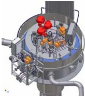
Small Column Ion Exchange module
