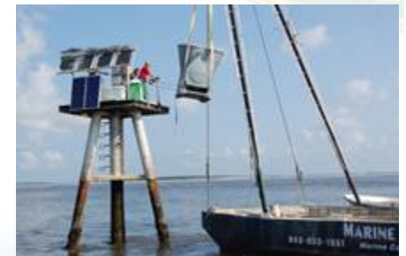
Testing SODAR to measure off-shore wind
