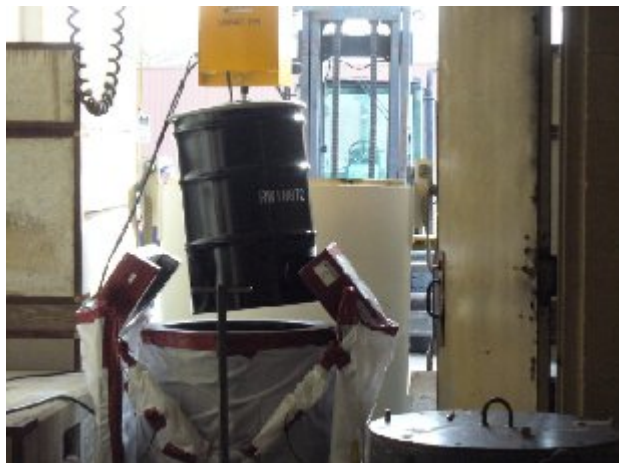
Fig. 5. RH-TRU drum being lifted/transferred from the gated drum shield.
