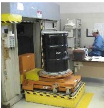
Fig. 2. Examination of the physical form of drum contents using RTR unit.
