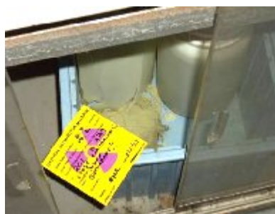
Fig. 6. Example of unneeded chemicals in containers that deteriorated over time and breached.
