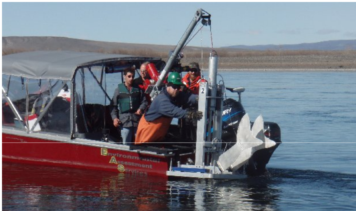
Fig. 3. Trident Probe Driving Frame and Rudder System for Deep and Fast-Moving Water.
