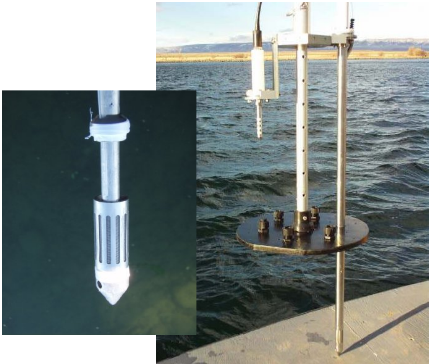
Fig. 2. Advanced Trident Probe Measurement and Sampling Tool and Closeup of Ruggedized Probe Tip. The pore water probe and surface water probe are configured for measurements approximately 30 cm into the riverbed and 30 cm above the riverbed, respectively.
