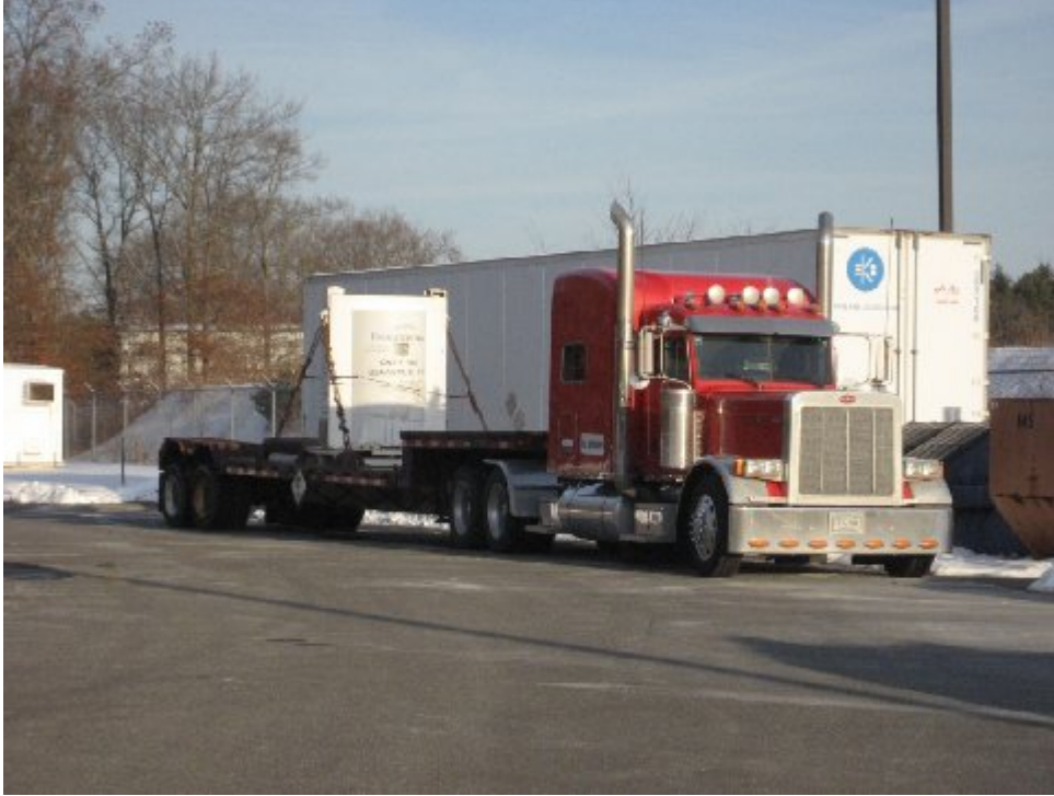
Figure 1 - Shipping Cask with Control Rod Blades Ready for the Road
