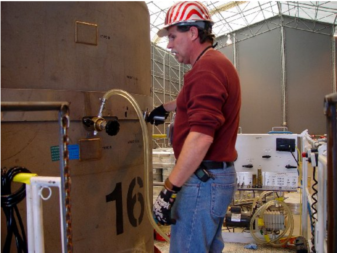
Fig. 2 Photograph of a leak testing TRUPACT II shipment.
