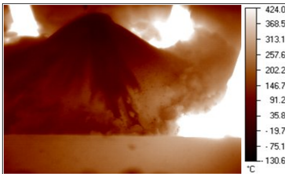
Fig. 3. Sellafield GeoMelt Treatment Trial 1 FWM Material
