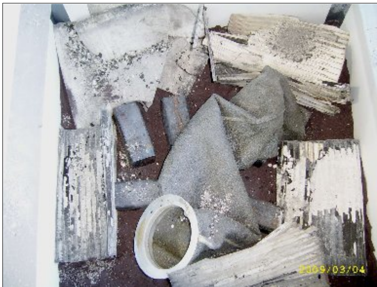
Fig. 6. Sellafield GeoMelt Trial 2 Steel Bar and Recycled Filters from Trial 1 as Waste Stream Simulant
