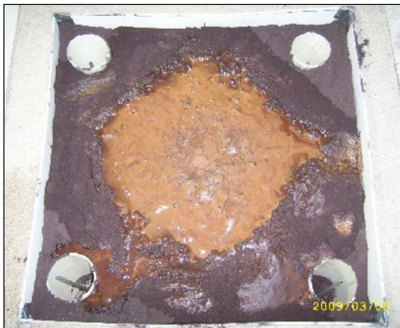
Fig. 7. Sellafield GeoMelt Trial 2 SIXEP Sand/Clino Waste Stream Simulant
