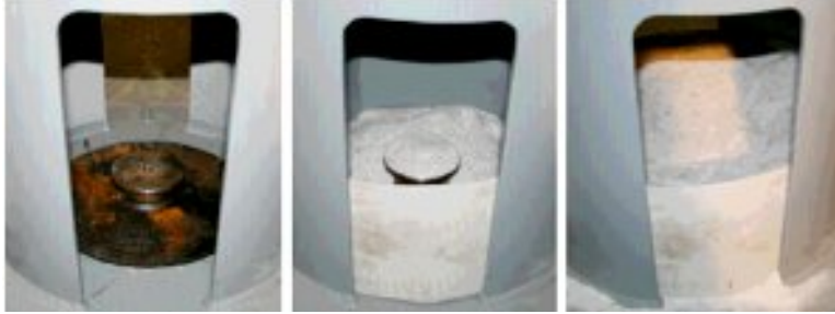
Fig. 9. Simulating crushed salt backfill before replacing the next canister
