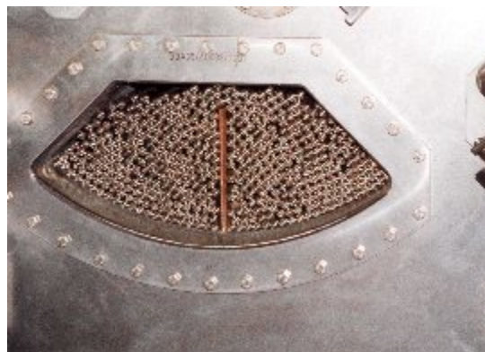
Fig.3. Fuel rods being loaded into one of a total of five POLLUX ® baskets
