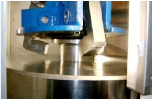
Fig. 10. Opening of the grab in the borehole
