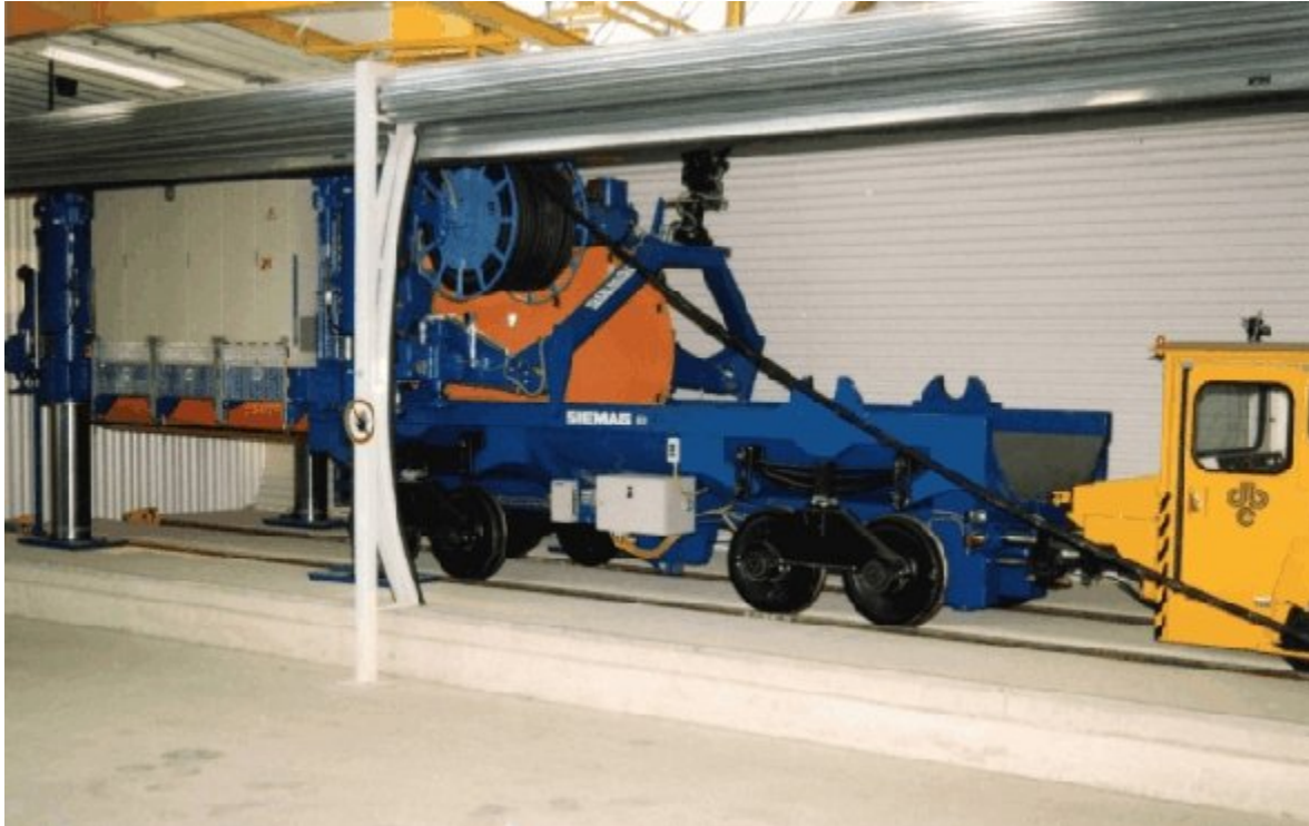
Fig. 6. Test facility with full-scale prototype of underground transportation and emplacement system
