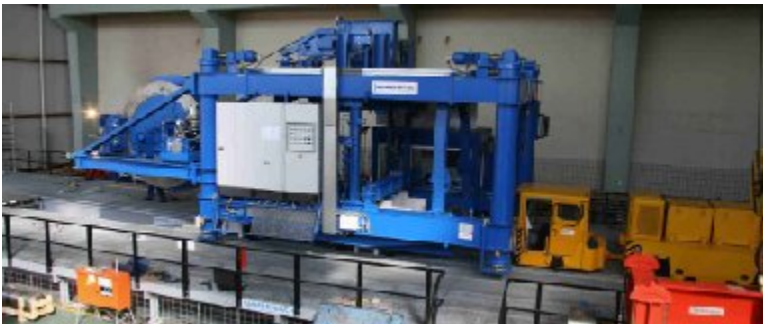
Fig. 11. Transport of the emplacement device by means of the transport cart
