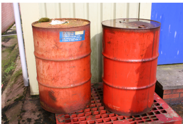
Fig. 4. Ad-hoc storage of organic waste at a Sellafield plant prior to recontainerisation and transfer to interim storage; showing degraded containers and insufficient bunded containment.
