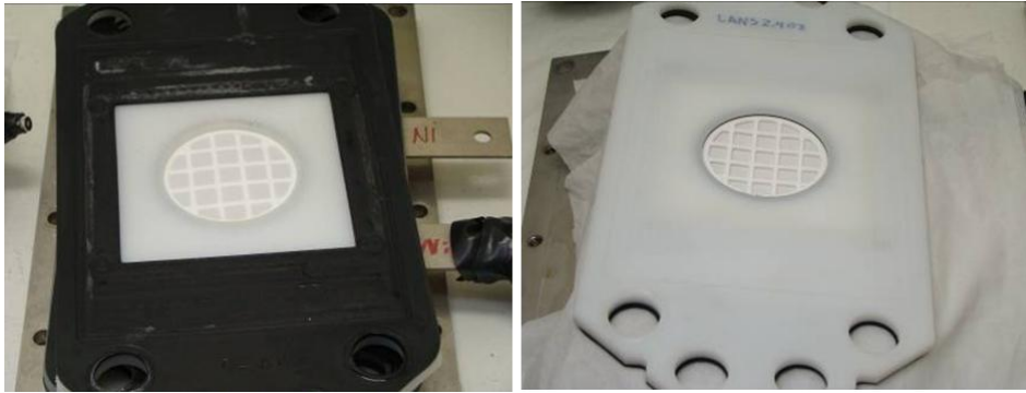
Figure 11: Post test optical image of the membrane: Anolyte side (left) and catholyte side (right)
