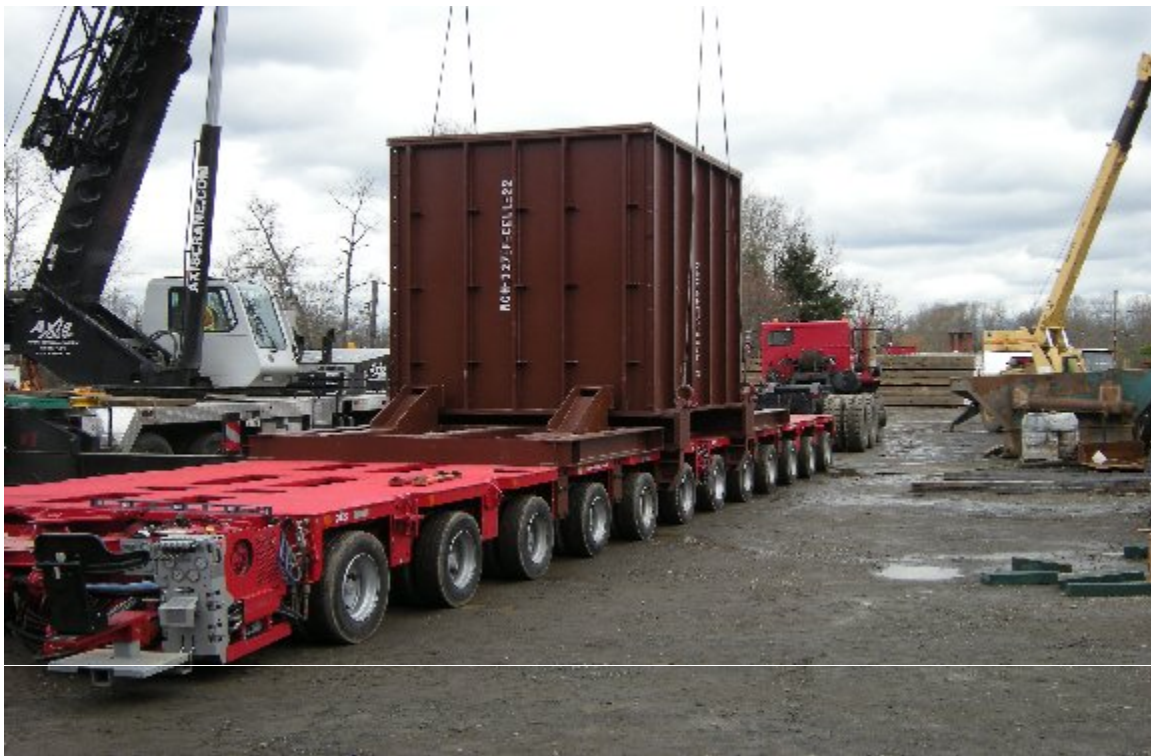
Figure 4. Packaged Hot Cell on Transporter
