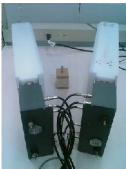
Figure 1 Two slab neutron counters in a “V” position ( \epsilon \sim 5.4\% ) and a Cf-252 source in the middle of the detectors inserted in a cardboard box.
