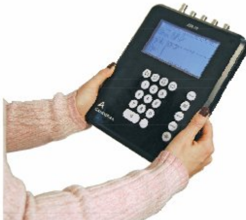
Figure 2 JSR-15 Hand Held Multiplicity Shift Register. There is a single shifter register input and two extra scalers. The JSR-15 weight is 1.7 kg and its dimensions are 254x203x32 mm
