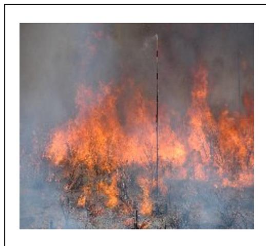
Fig. 1. Painted Fire Pole in Foreground Showing Thermocouple Mounted Perpendicular to the Pole at a Height of 2 m.
