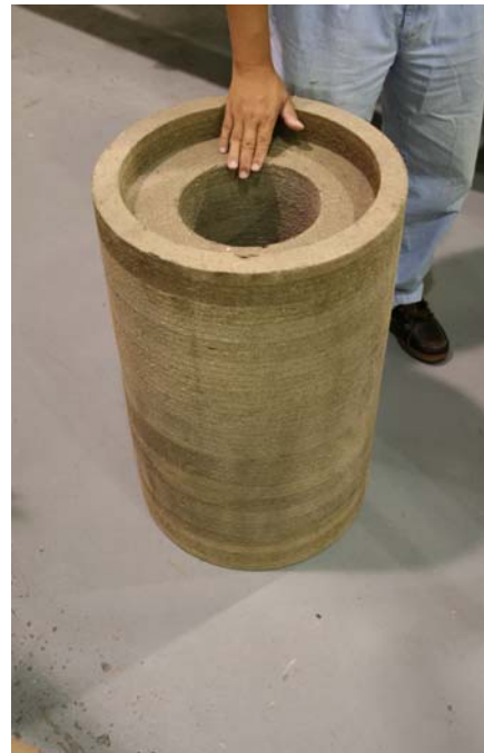
Figure 1. A Picture of a Model 9975 Shipping Package with cutaway and the 9975 Lower Celotex™ Assembly.
