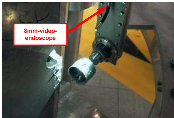
Fig. 4: Testing the milling device
