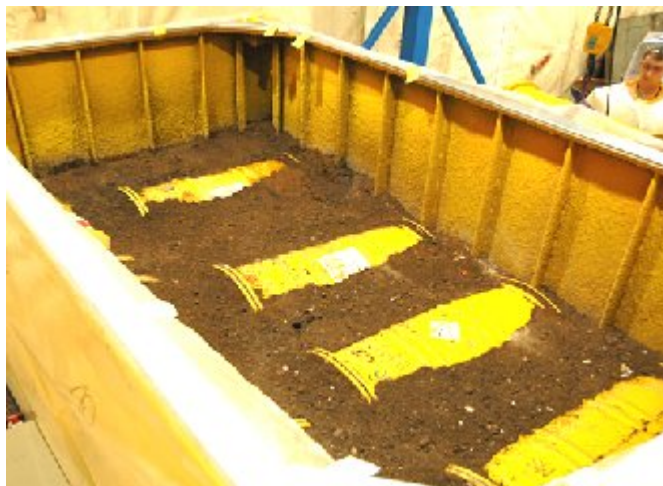
Figure 1: Filling of containers with drums and debris
