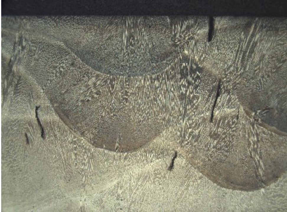
Fig. 3. Magnified cross section of a Haynes 556 weld coupon showing microfissures.
