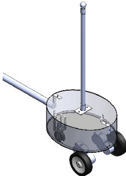
Fig. 3. Mobile platform with PVC pipe and nozzle attached.
