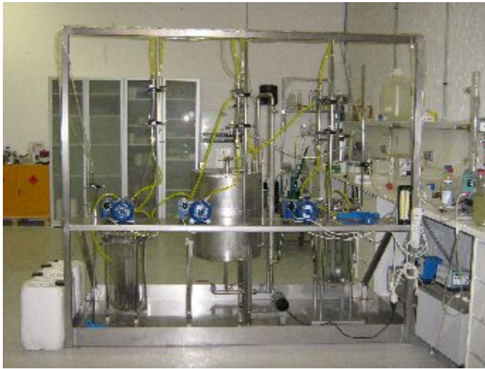
Figure 2: Picture of the digester and cross flow filters
