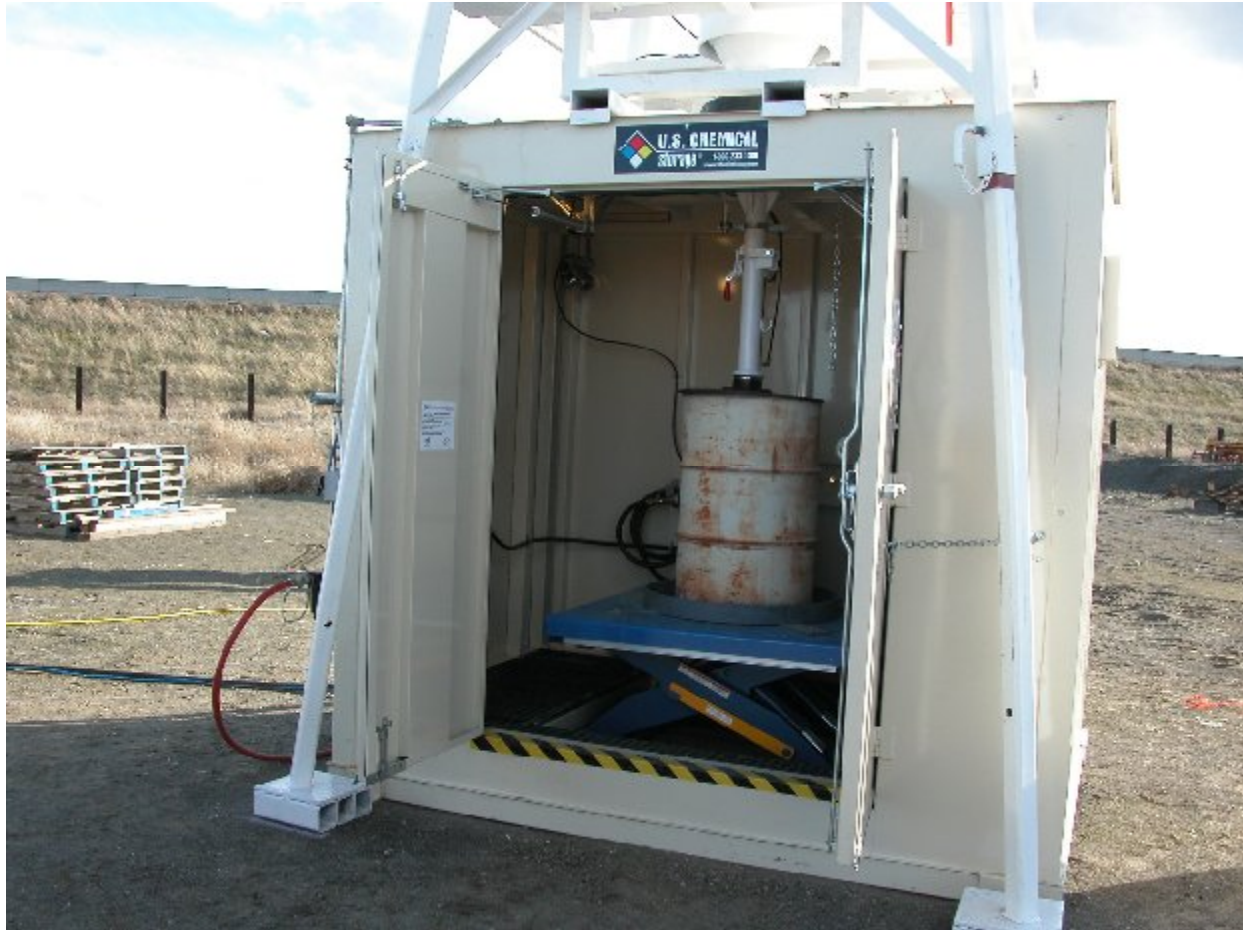
Fig. 4. Pre-project testing of the drum punch facility using an empty drum.
