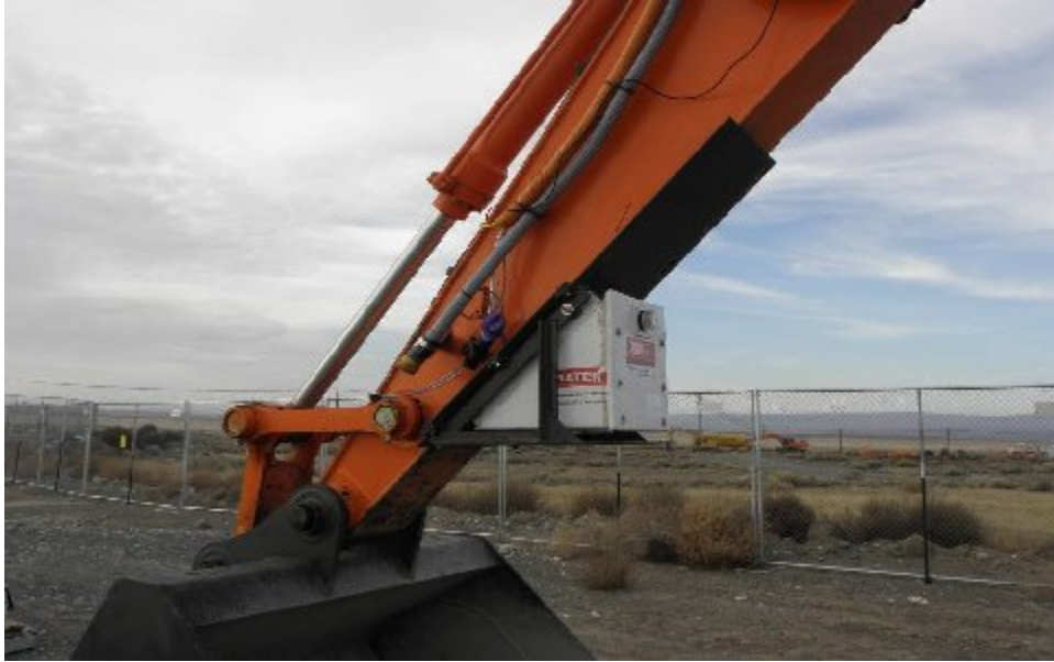
Fig. 2. CRATER™ Redesigned Brackets on Excavator Boom
