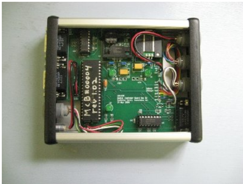
Figure #6 Master Controller Board with Top Removed
