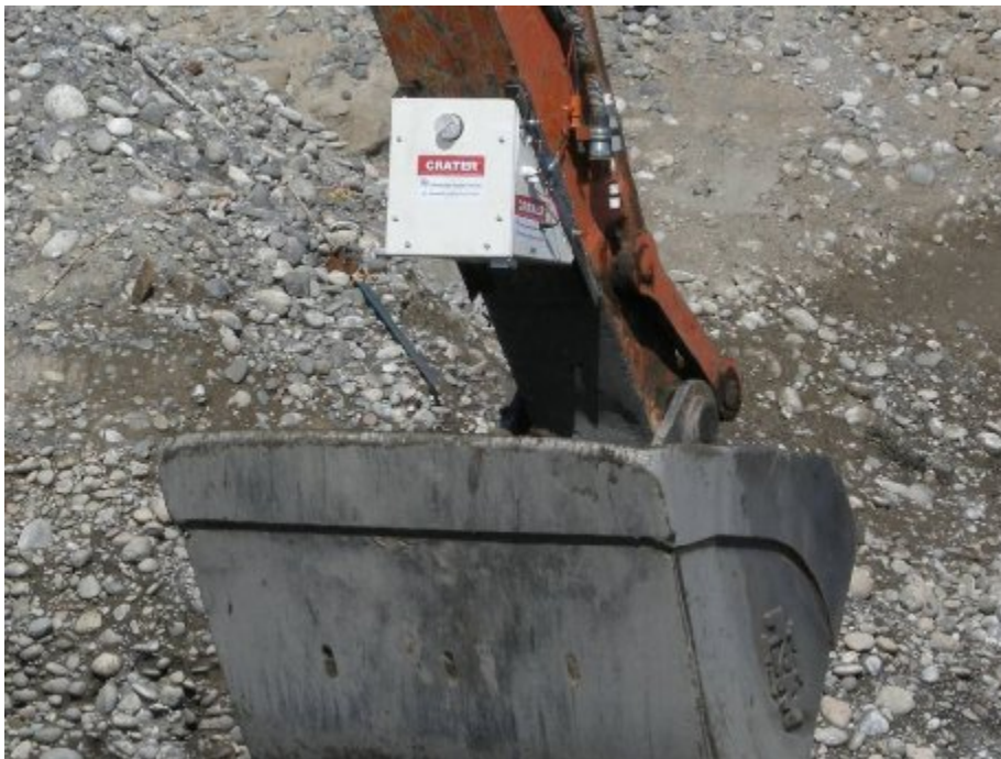
Fig. 1. CRATER™ Original Bracket on Excavator Boom
