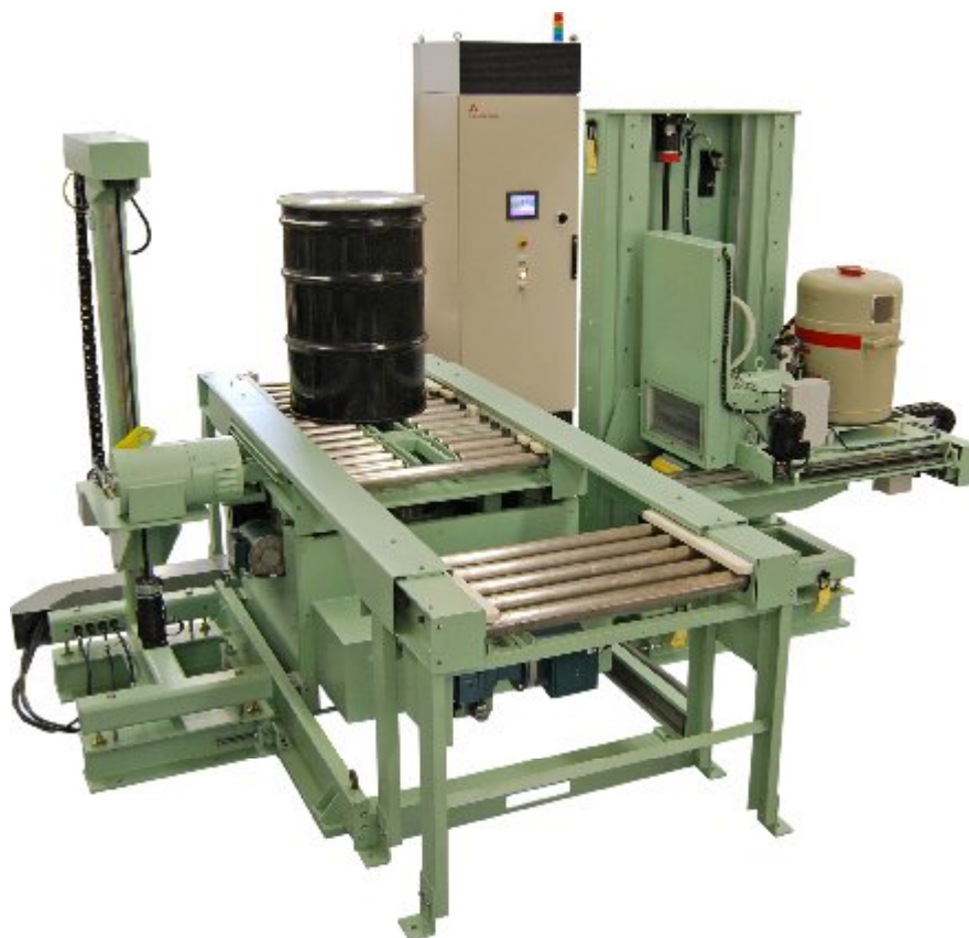
Figure 1. Photograph of the industrial TGS system during factory assembly. The transmission assembly is viewable on the left. To the right is the germanium detector and surrounding aperture box. The drum is shown on the in-feed conveyor.
