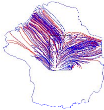
(b) Trajectories of water particle for future environmental conditions (80,000 years later) (Case 2)
