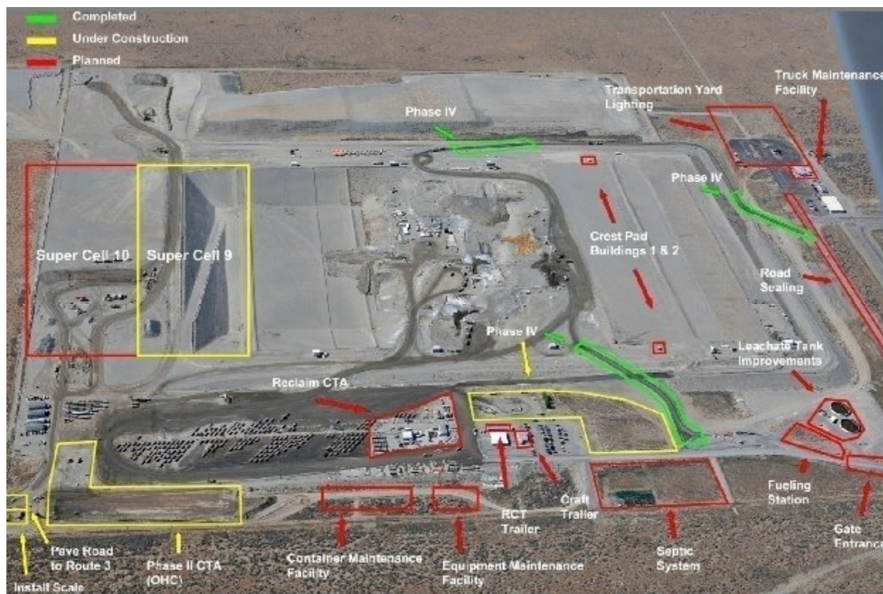
Figure 4. ARRA-funded work at ERDF is being completed in several phases. The facility upgrades and expansions are designed to accommodate significantly increased waste volumes over the next several years, as identified by waste generators.
