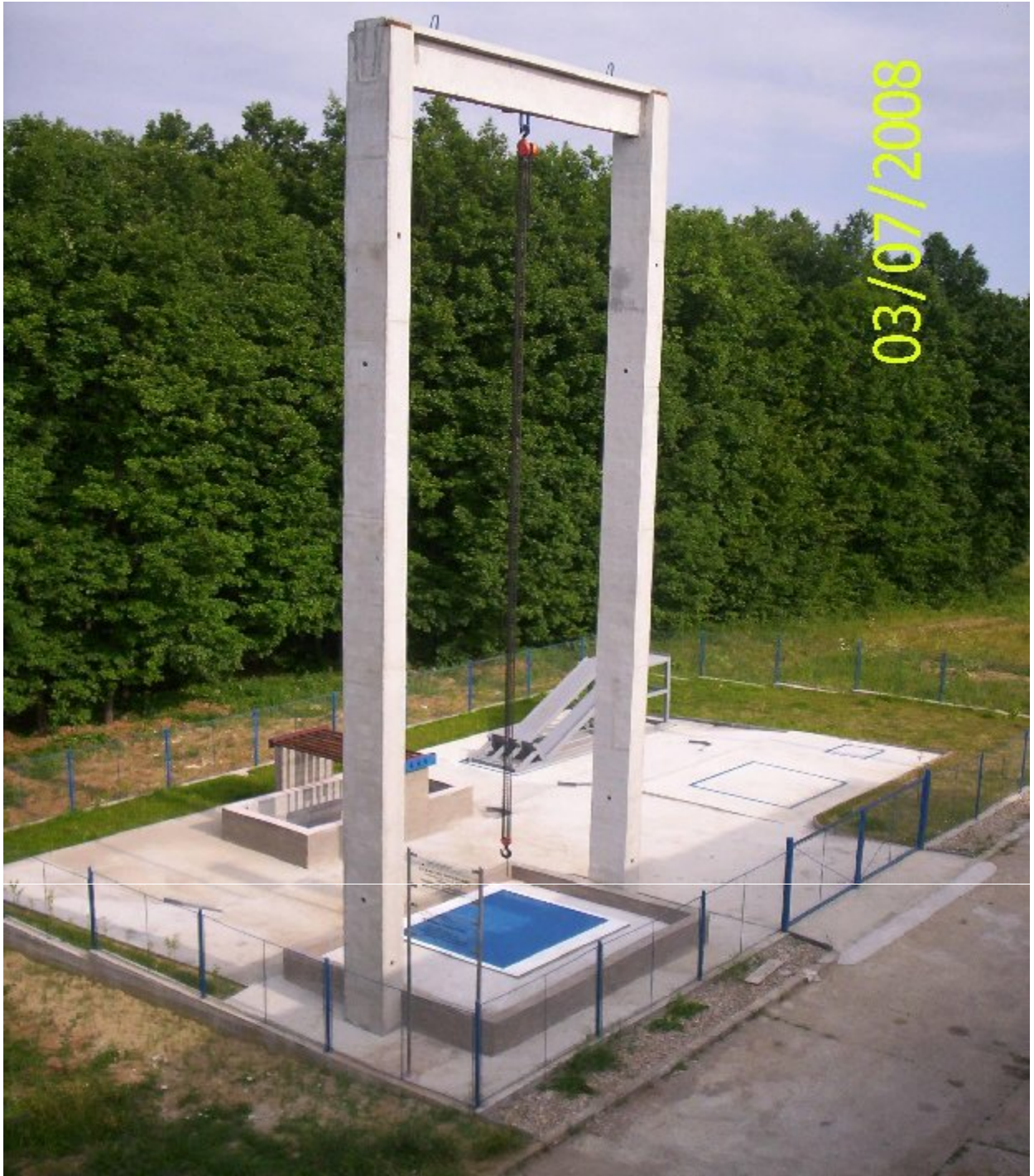
Figure 2 – An overview of the New Romanian Testing Facility for Type A, B and C packages.
