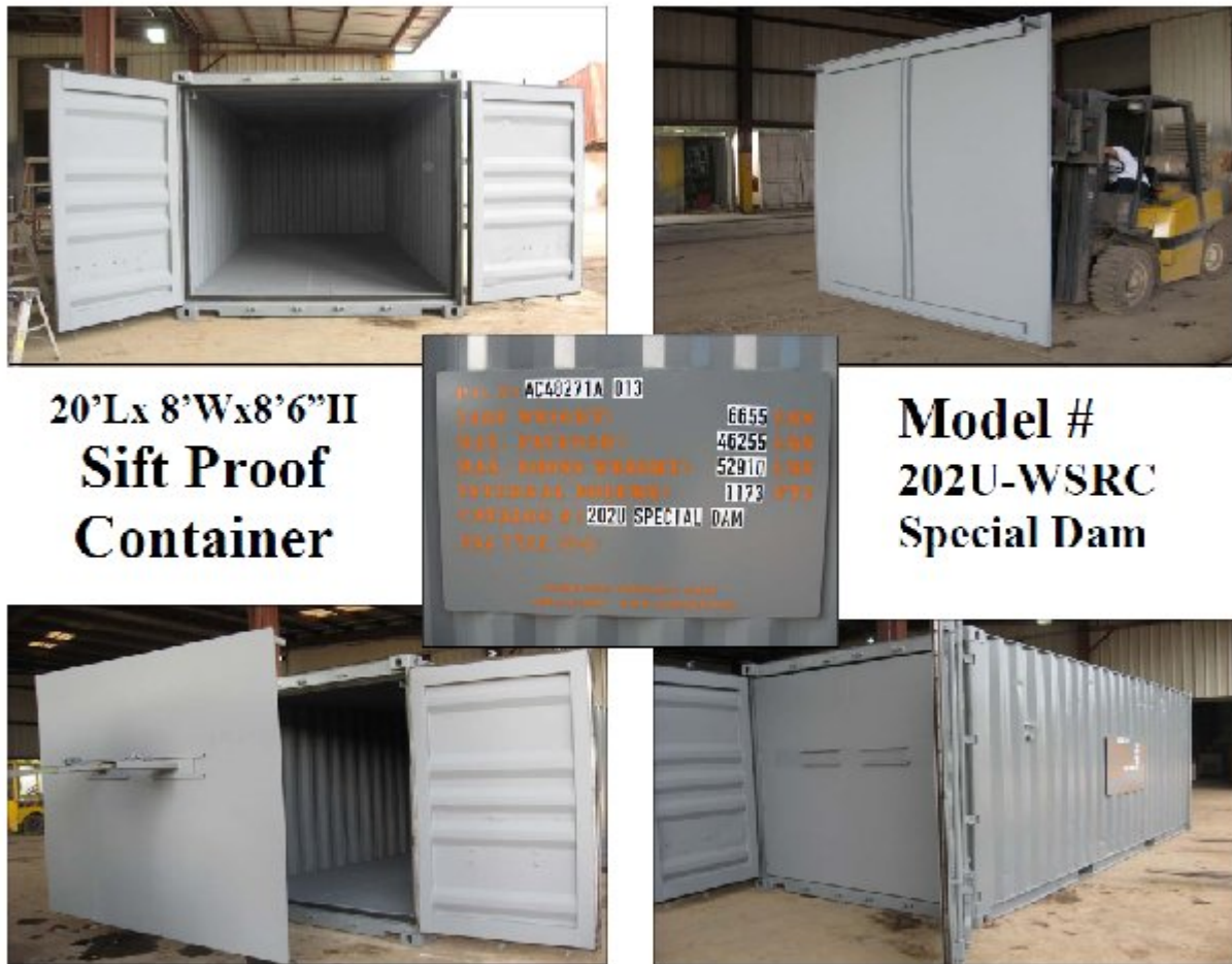
Fig. 3. Sift-proof containers from Savannah River Site.
