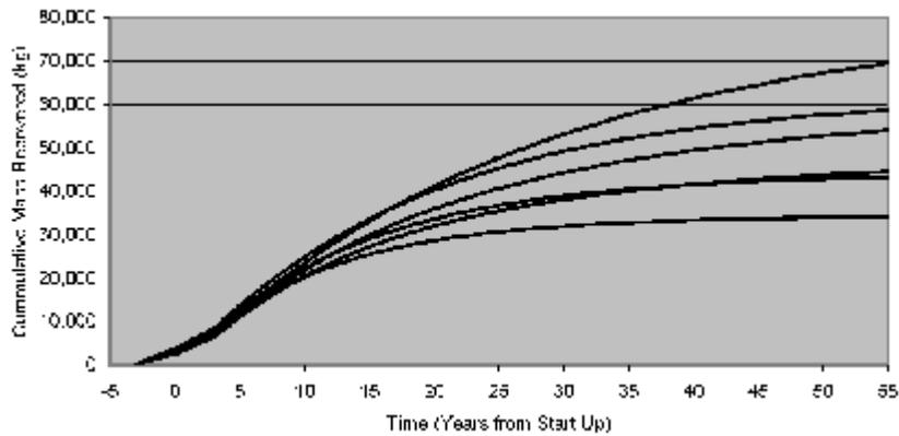
Figure 4. Percent of Dissolved Carbon Tetrachloride Mass Recovered (Extracted and Treated): Maximum and Minimum Calculated.
