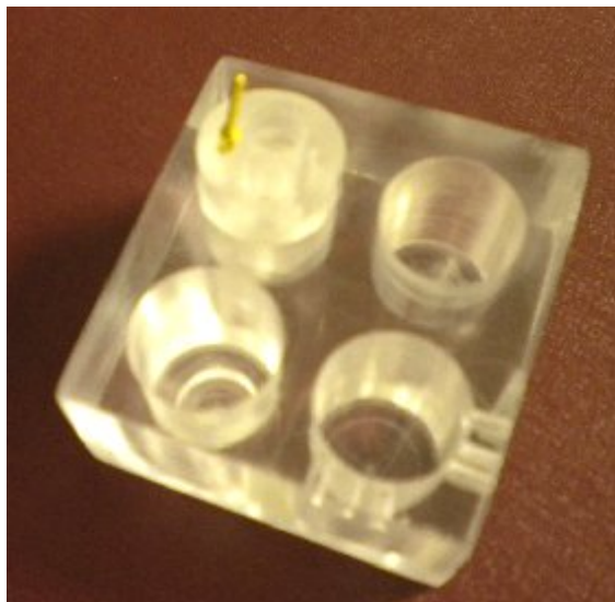
Fig. 1. The custom-made micro electrochemical measuring cell.
