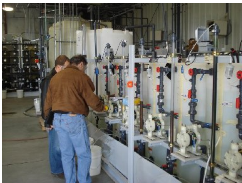
Fig. 3. Resin Test Skid in Operation
