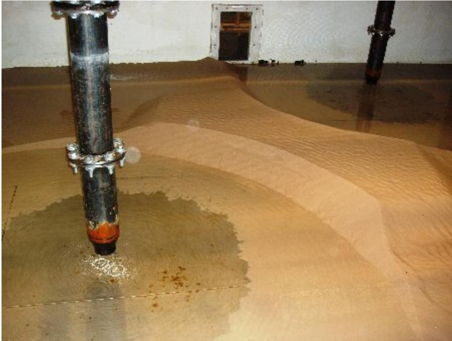
Fig. 10: Sand inside flume after testing clearly showing the ZOI of the jets
