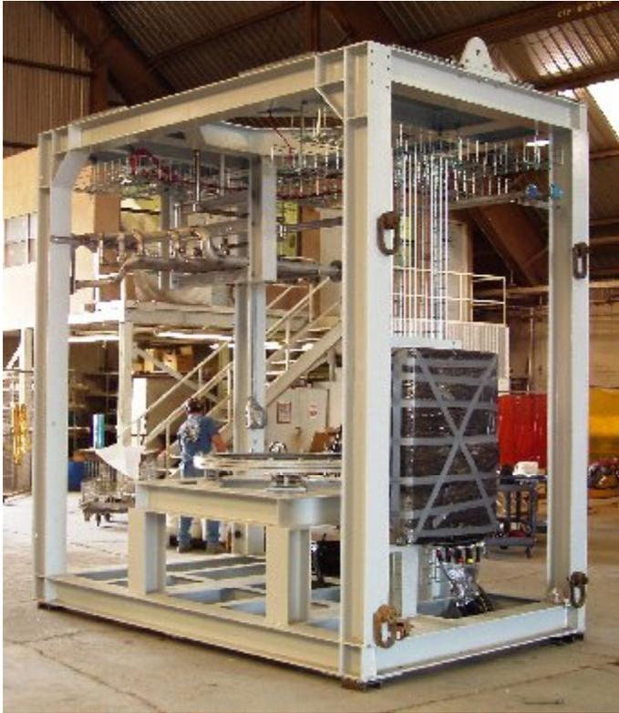
Fig. 4: Test vessel #2 skid (P2) showing the lower mounting ring for the acrylic vessel
