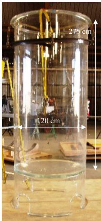
Fig. 2: 1.2m diameter acrylic test vessel
