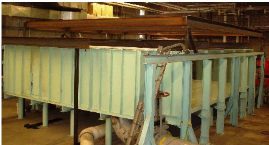
Fig. 8: Radial flume vessel during construction
