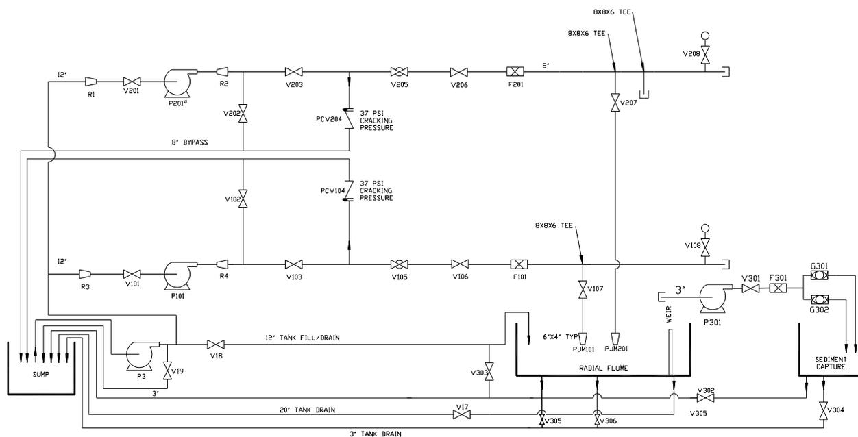
Fig. 7: PFD for Radial Flume at WSU
