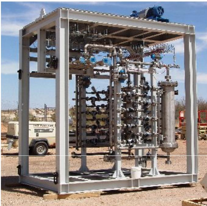
Fig. 5: PJM control valve rack skid (P3) ready for shipping
