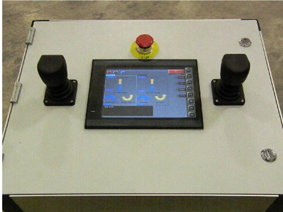
Figure 3: Dual-Joystick Control Console
