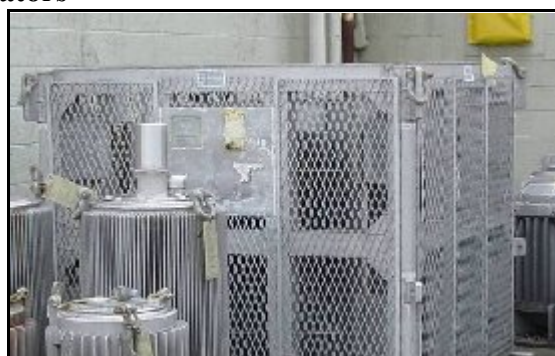
Fig. 3. Radioisotope thermoelectric generator.
