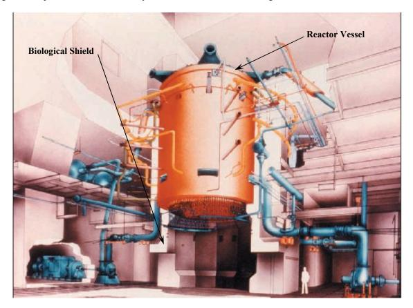
Figure 1. SRS Heavy Water Reactor [2].
