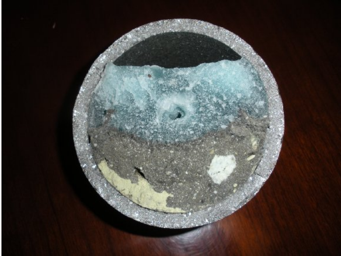
Fig. 2. Waxfix Penetrated through the Dry Cement to Fix the Bottom Layer of Dusting Sulfur.
