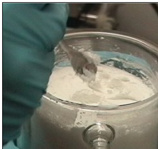
Fig. 4. Photograph of filter cake texture.
