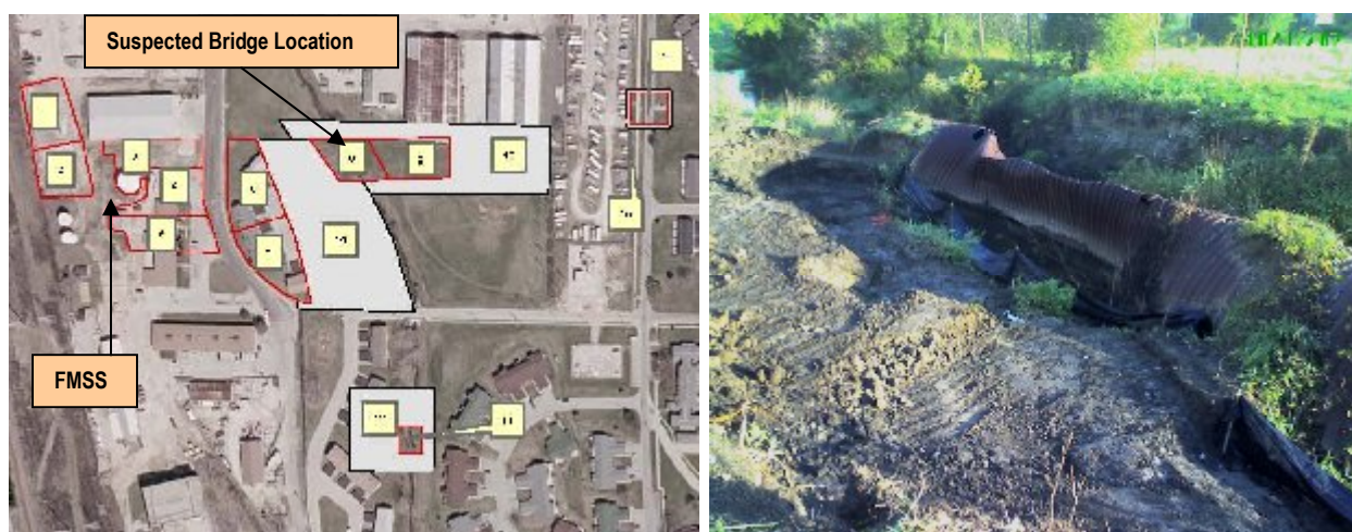
Fig. 4. Map of All FMSSA Impacted Areas at NSGL and a Photo of Corrugated Metal Culvert Pipe in Skokie Creek where Suspected Bridge Would Have Been Located.
