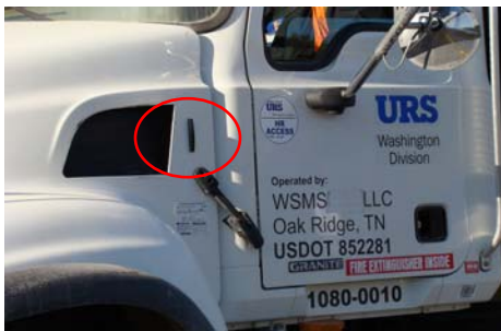
Figure 2 Passive RFID tag mounted on Truck
