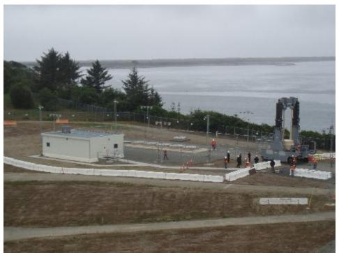
Figure 17 - The VCT Entering the ISFSI Security Area with a Loaded HI-STAR HB
