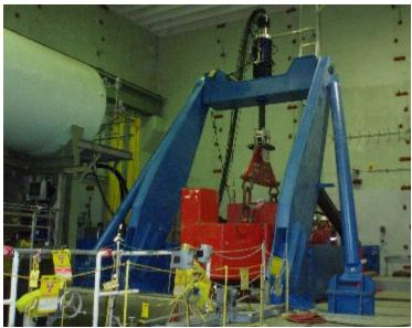
Figure 11 - Post-Installation Load Test of the Davit Crane
