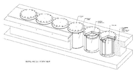
Figure 4 - Isometric View of ISFSI Vault
