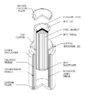
Figure 8 - HI-STAR HB with MPC Partially Inserted
