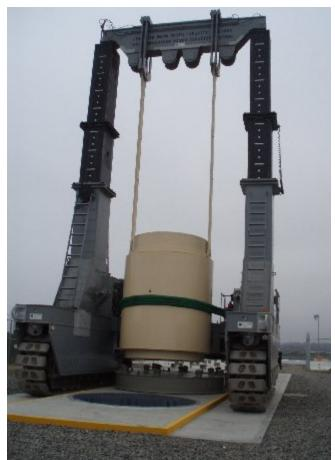
Figure 18 - VCT Preparing to Lower a HI-STAR HB into the ISFSI Vault
