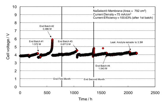
Fig.7. Cell Voltage Change during Three-Month Batch Recycle Mode Test
