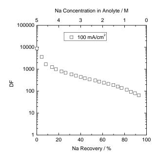
Fig. 10. Na Recovery vs DF of Cs-137 Resulting from Test at 100 mA/cm<sup>2</sup>
