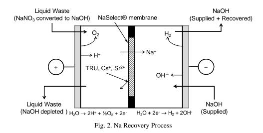
Key issues in the sodium ion recovery process are as follows:
