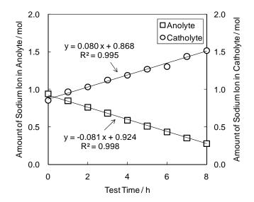
Fig. 5. Sodium Ion Transport Rate during Test
