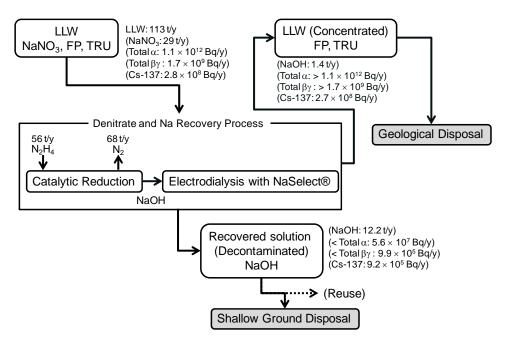
Fig. 11. Material Balance by the DNR process
