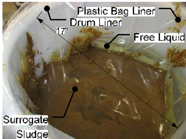
Figure 3. 200,000 cP surrogate sludge plus 2.6-gallons of free liquid.
