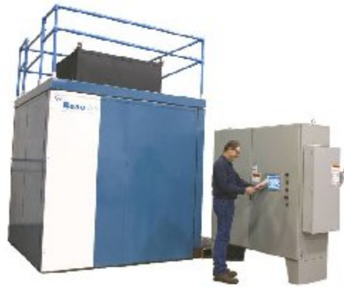
Figure 1. Resodyn 30-gallon industrial scale ResonantAcoustic ® Mixer.
