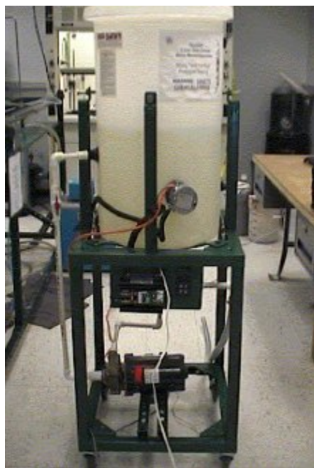
Figure 7. The slurry tank used during steady state tests. It has SCR-controlled heaters for temperature control and a pumping system that keeps the slurry well mixed by drawing slurry from the top and pumping it through the pump bottom.
