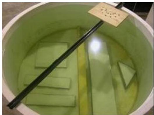
Figure 10. 6 ft plastic tank with 5 metal forms filled with plastic beads of density 1.04 \text{ g/cc} .
