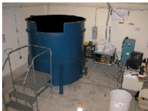
Figure 8. FIU Test Tank (7-ft 2-in diameter) for the Solid Liquid Interface Monitor (SLIM).
