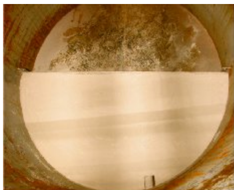
Figure 9. Kaolin Clay in tank configured to take up half of tank bottom.
