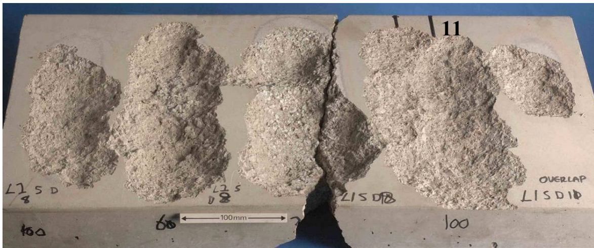
Fig. 9. The scabbling process on concrete containing limestone aggregate: Run 11 - double side by side pass, each at 100mm/min.
