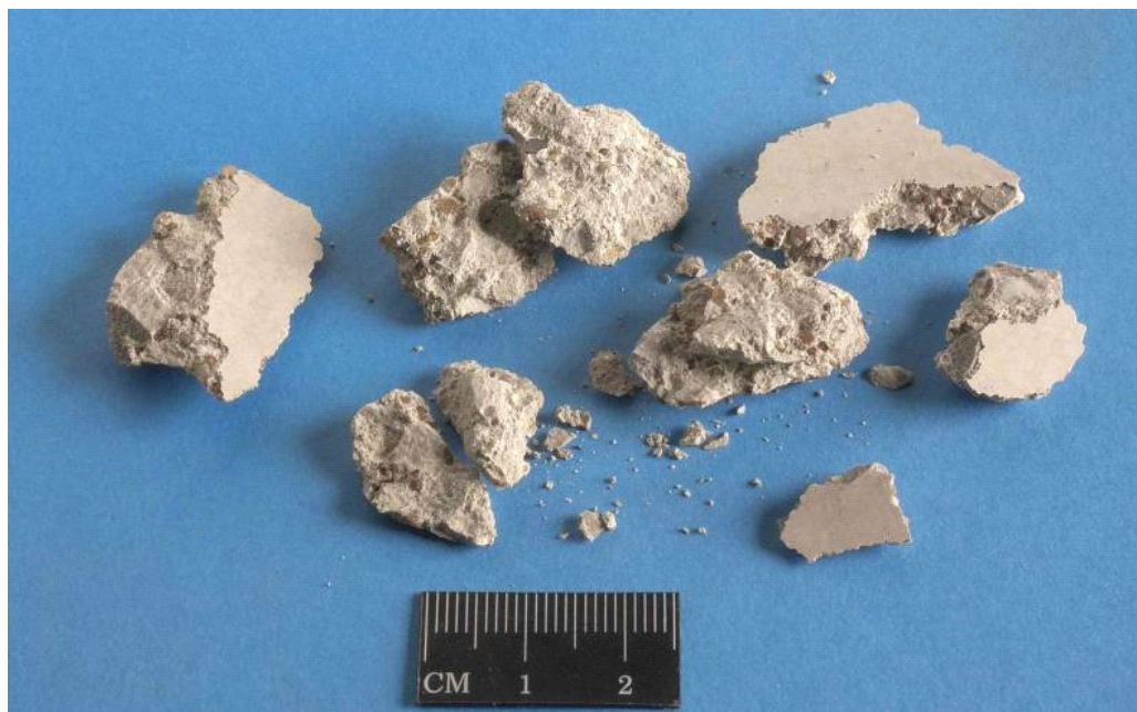
Fig. 7. Typical debris from the scabbling process on limestone aggregate concrete.
