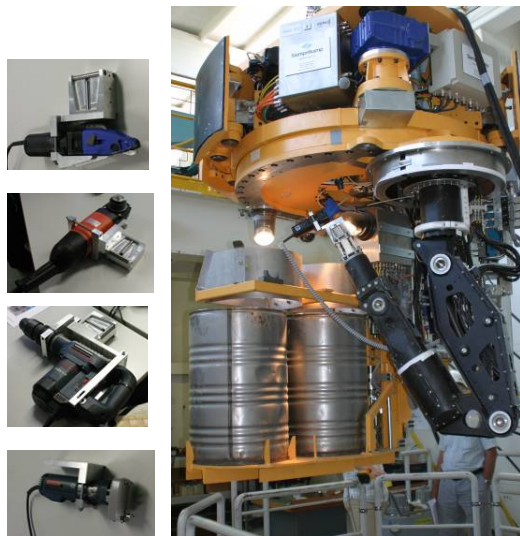
Figure 2: Tool carrier system with manipulator system and working tools
