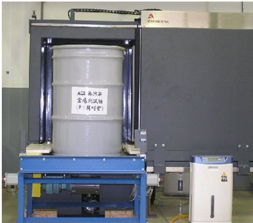
Fig. 2. CAS system at INER. This view shows the drum in the load/unload position and the AQ2 system in the background with the sliding shield door open.
