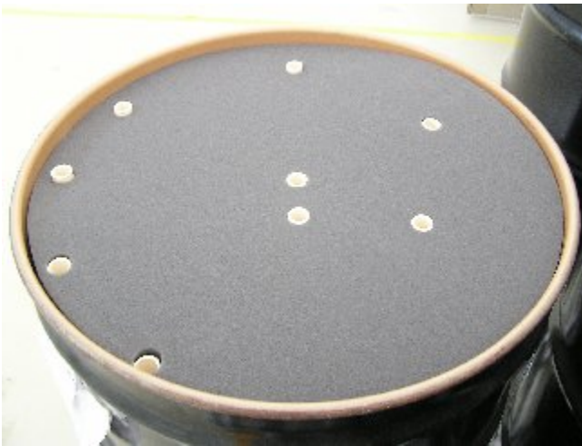
Fig. 1. A simulated standard drum used for efficiency calibration with method 1.
