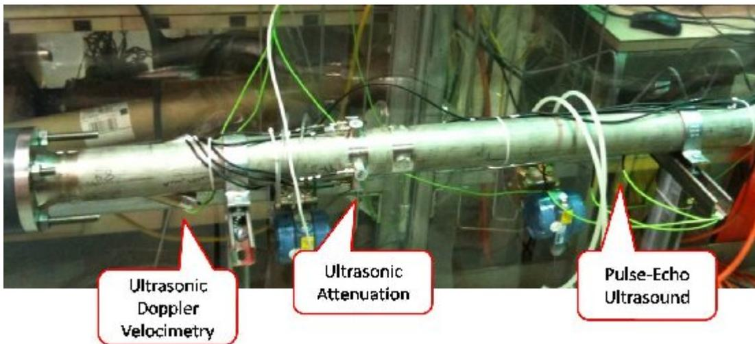
Figure 8. Instrument Test Section
