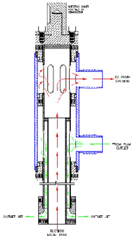
Figure 2. Scaled Mixer Pump Details
