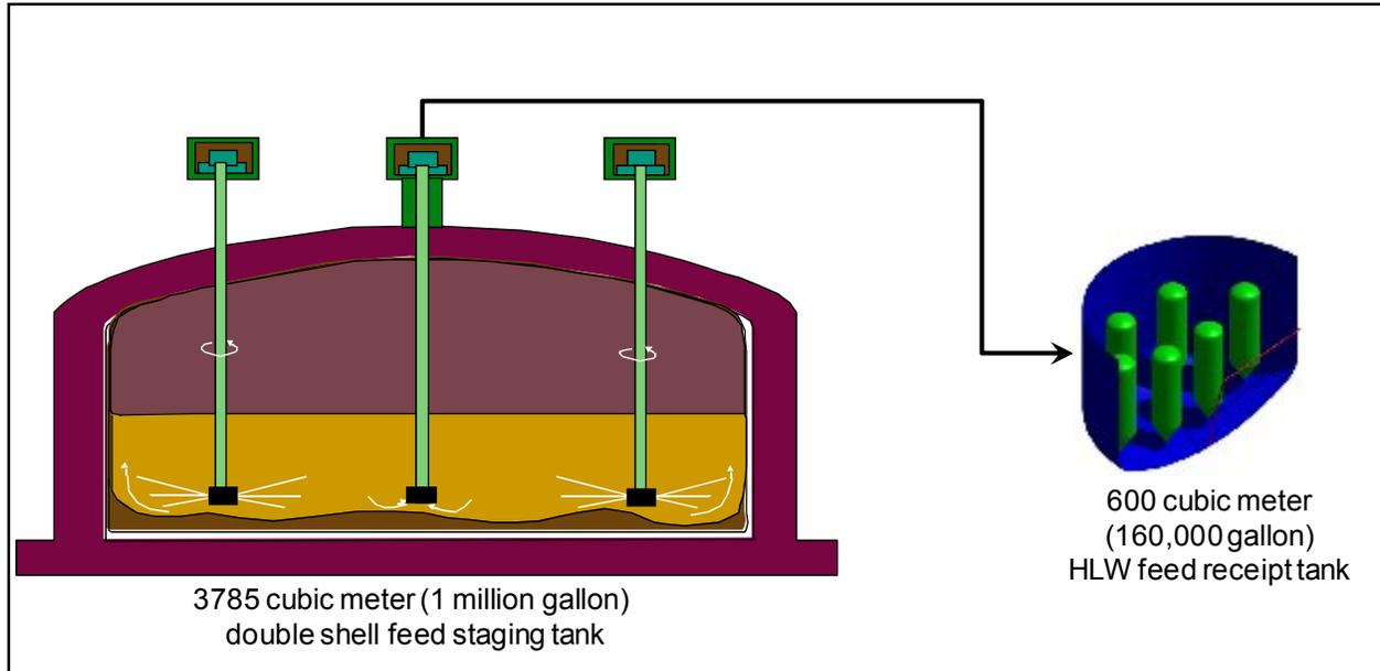
Figure 1. WTP Feed Delivery Concept
