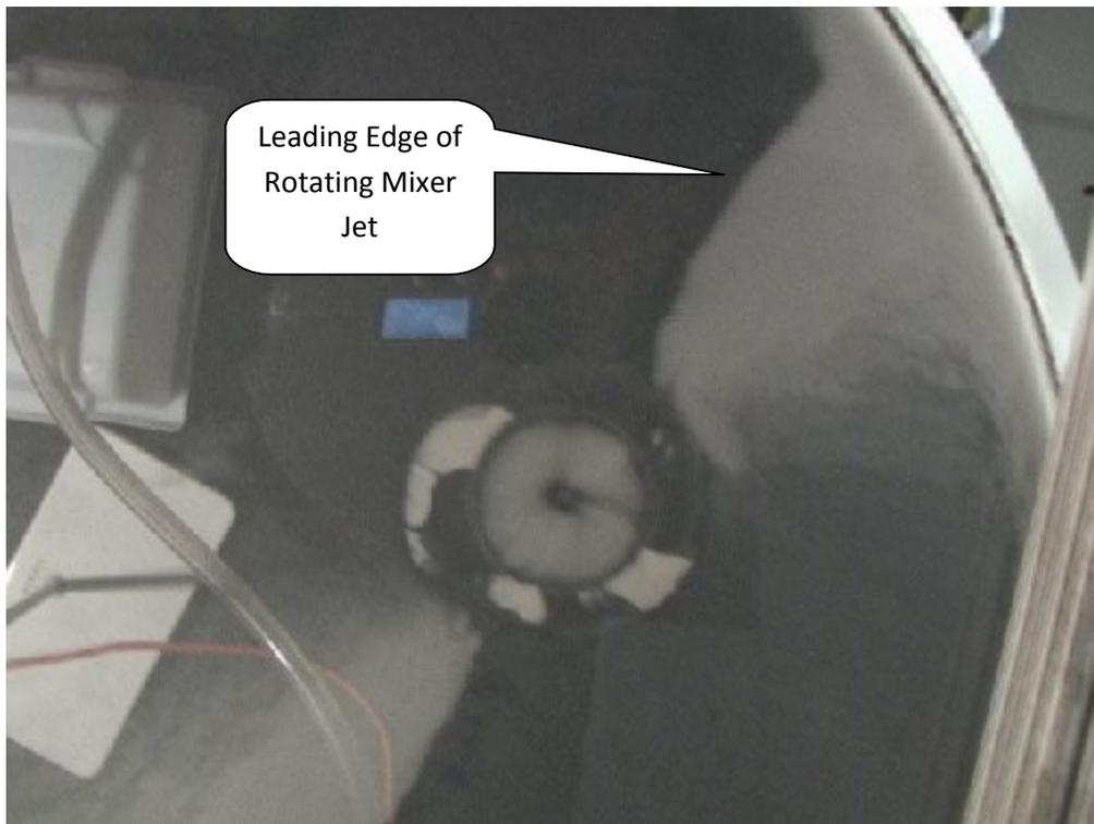
Figure 4. Mixer Pump Clearing of Tank Bottom
